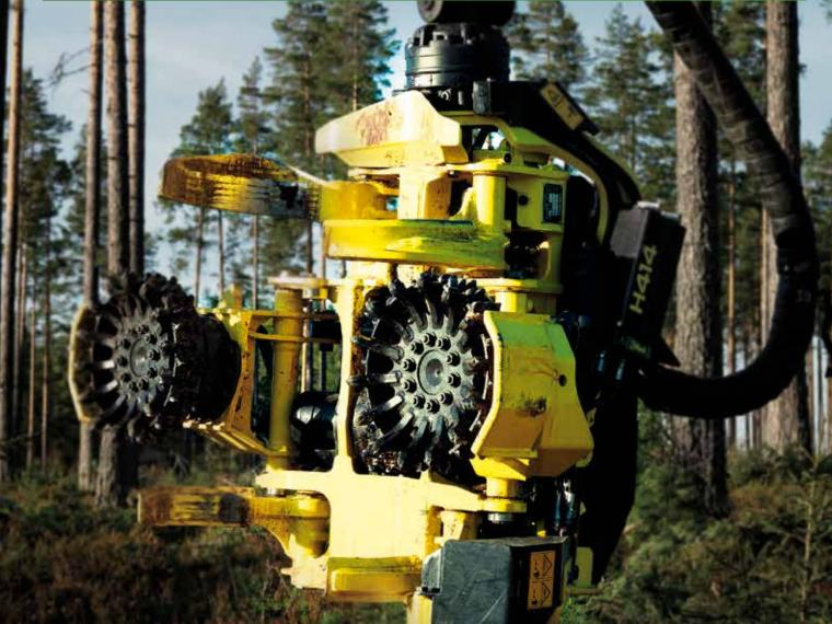
Feed-roller arms feature built-in guards, strong cylinders and well-protected hose routings. Four moving delimbing knives, one fixed top knife, and one fixed back knife follow the contours of the stem.
