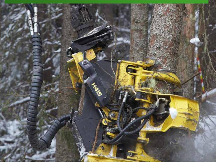
The H415 gives unprecedented tree-processing performance, especially in large timber. New feed-roller-arm geometry ensures feed rollers grip solidly and reliably carry trunks in all diameter ranges.
